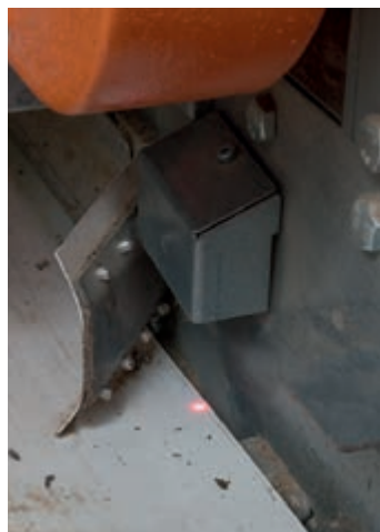
Light sensors monitor the belts
