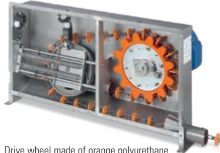
Drive wheel made of orange polyurethane
