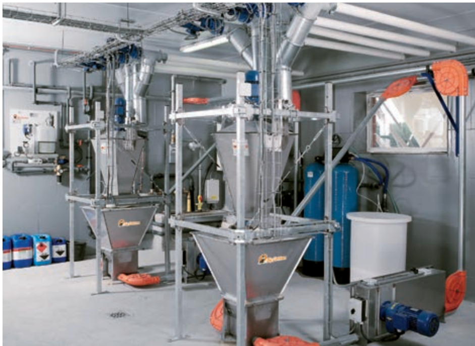
DryExact pro feed kitchen: two systems with one circuit each
