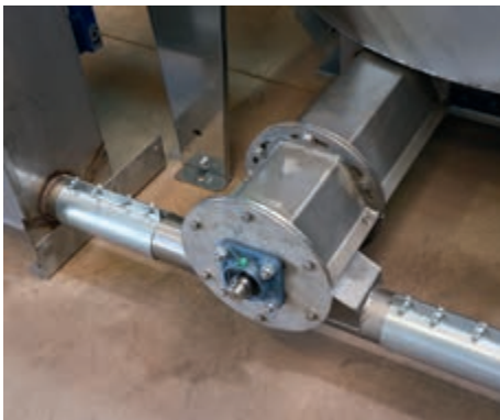
Special transfer unit between the dispenser's discharging auger and the DR 1500 pipe conveying system
